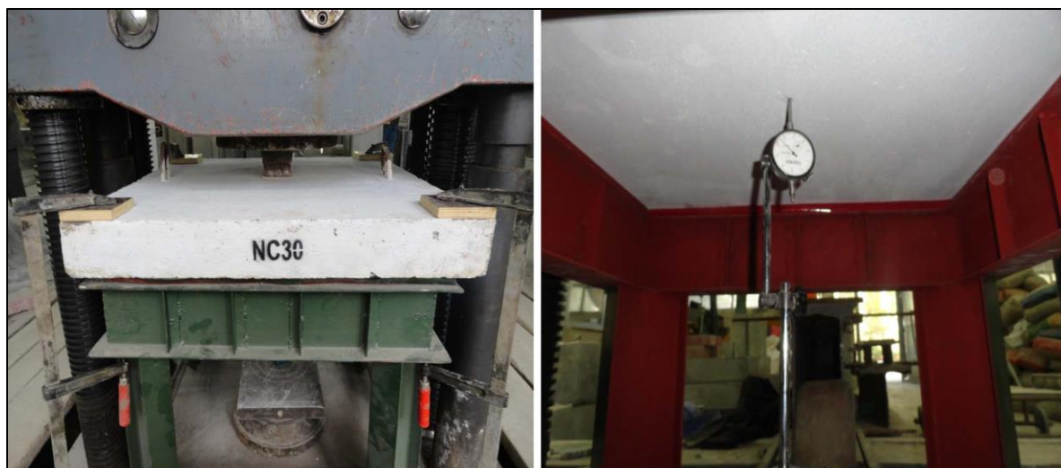
Fig. (4): Test set-up of slabs.
